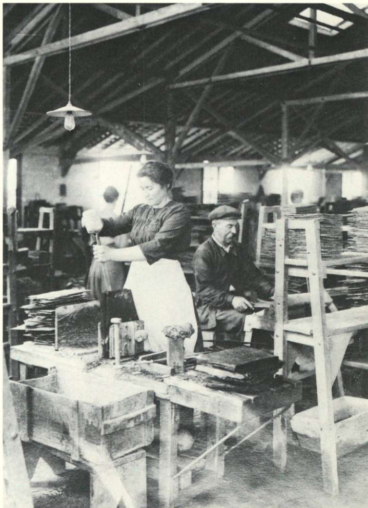
Under a bare bulb, with chisel and mallet, a Welsh slatemaker splits the stone into thin pieces. The man seated behind her works at a slate-trimming machine. Photo, c. 1900. Courtesy Welsh Room, Green Mountain College Library, Poultney.
