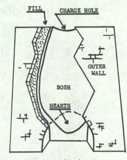
Cutaway view into a typical blast furnace.
