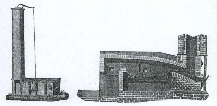
Figure 15. Puddling furnace elevation (left) and vertical section (right). Notice similarity to figure 9 (Overman 1850:260, 264).
