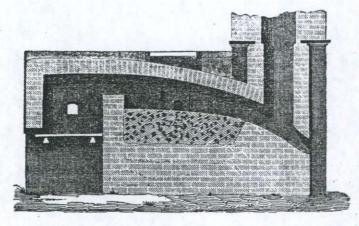
Figure 9. A section through a reheating furnace (Overman 1850:372).
