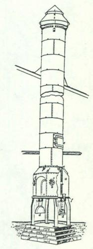
This, too, is an iron furnace—a cupola found in old foundries, where it was used to melt pig and scrap iron for casting; it was built around 1900.
