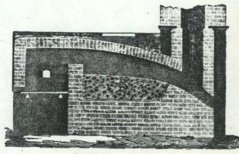
Section of a re-heating furnace.
