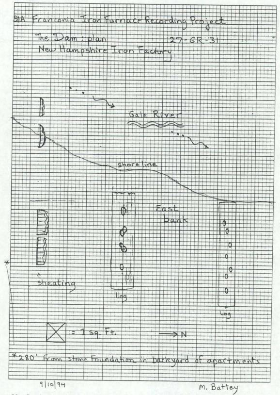
Figure 39. Surface remains of cribbing at the dam site (Megan Battey field sketch).
