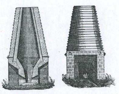
Figure 4. A section and interior (left), and front view (right) of a cupola blast furnace (Overman 1850:163).
