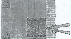
Figure 11. Vertical section of bloomery fire (top); plan at hearth level (bottom). Hearth at point "a" (Overman 1850: 246).
