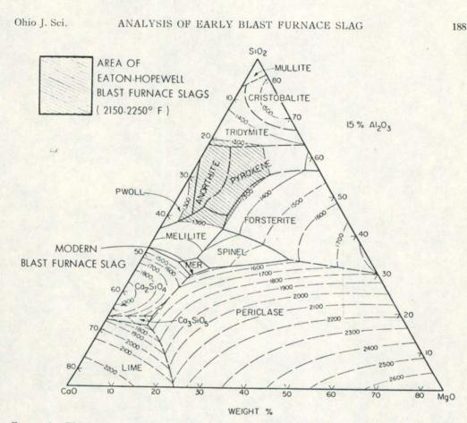
FIGURE 1. Phase relations at liquidus temperatures in the 15% Al<sub>2</sub>O<sub>3</sub> plane of the CaO-MgO-Al<sub>2</sub>O<sub>3</sub>-SiO<sub>2</sub> system, showing position of Eaton-Hopewell Furnace slags in relation to those of a modern blast furnace. Temperature in degrees Celcius.
