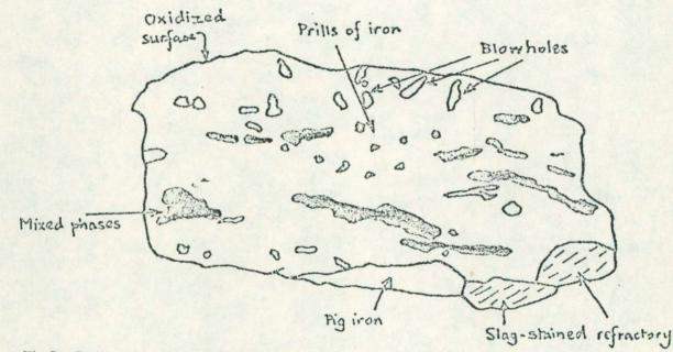
Fig. 5 - Section through Cannock cinder
