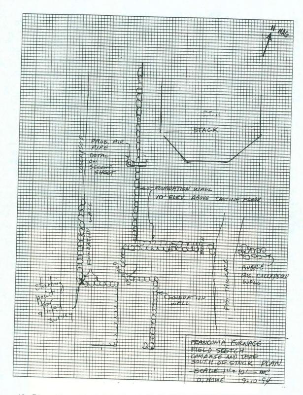
Figure 46. Disposition of the foundation walls with respect to the furnace stack (Dennis Howe field sketch).
