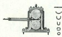
Figure 2. The barrel rolling and welding mill as used at Springfield and other New England Armories in the mid-19th century. The skelp of bar iron is bent up by successive passes through grooved rolls as above on the right and then welded between rolls and a stationary mandrel, as shown on the left. Courtesy of Robert Gordon.
