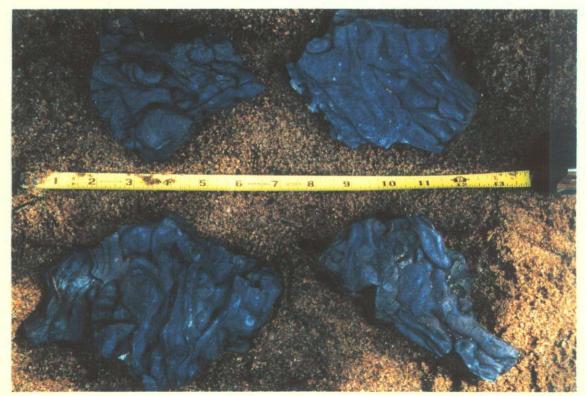
Figure E2. Possible bloomery "tap slag" or puddling slag (Matt Kierstead photo).
