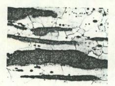
Figure 1. Photographs at the same magnification of the structure of a sample of bar iron made (left) in Litchfield County (Connecticut) and (right) at Marshall's works, Wednesbury, England. The English iron has much finer and more uniformly distributed slag particles. Courtesy of Robert Gordon.
