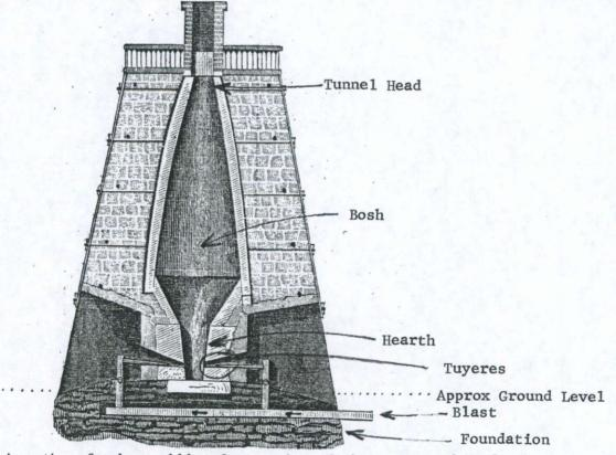
Figure 1. A section of a charcoal blast furnace through the tuyere arches (Overman 1850:153).
