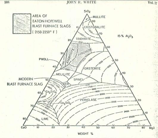
FIGURE 1. Phase relations at liquidus temperatures in the 15% Al<sub>2</sub>O<sub>3</sub> plane of the CaO-MgO-Al<sub>2</sub>O<sub>3</sub>-SiO<sub>2</sub> system, showing position of Eaton-Hopewell Furnace slags in relation to those of a modern blast furnace. Temperature in degrees Celcius.
