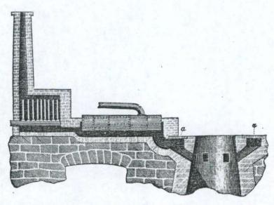
Figure 3. A hot blast oven atop the blast furnace stack, showing how hot exhaust gas was tapped (Overman 1850:450).
