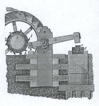
Figure 12. Tilt hammer and foundation pilings (left) and helve ring (center). The helve ring served as the strong fulcrum on which the full weight of the helve rested (Overman 1850:335).
