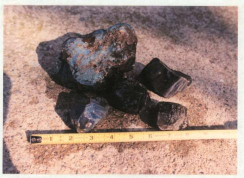
Figure 37. Typical pieces of blast furnace slag found at the site.
