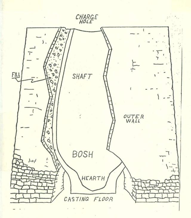
A cutaway view of an early blast furnace, similar to most pre-Civil War blast furnaces in Vermont.
