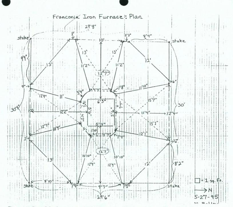
Figure 14. Ground-level measurements of arch openings, hearth, and corner pillars (Megan Battey field sketch).
