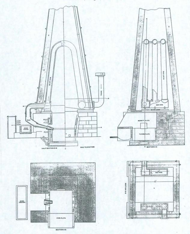
Figure 13. A three-pipe variety Champlain Forge, used at Saranac, New York, but typical of that which operated at East Middlebury (Egleston Sept. 1879: plate 4).
