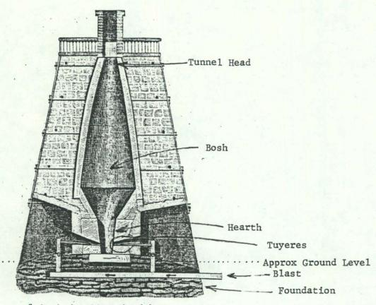
Section of a charcoal furnace through the tuyere arches.
